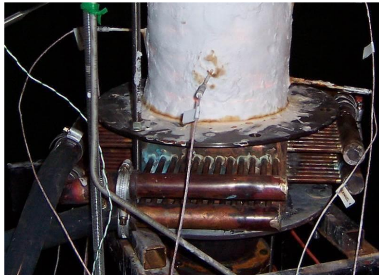
Figure 5.3: Photograph of the heat exchanger assembly
