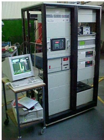
Figure 3.6: Gas analyser system showing the different analysers and data acquisition system
