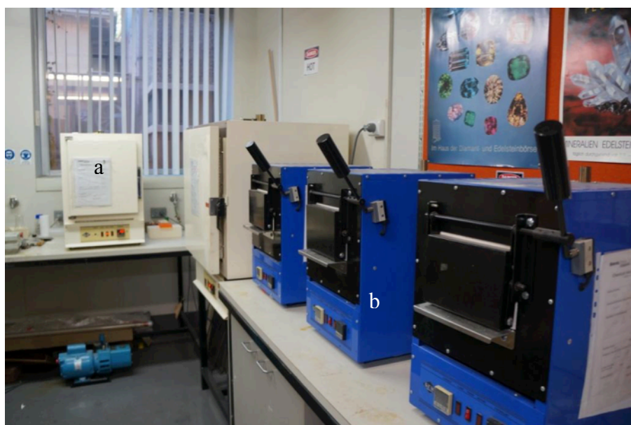
Figure 2.3 ovens (a) and Muffle furnaces (b) used in this work. These furnaces/ovens are programmable and the temperature can be controlled precisely with \pm 2 °C. The maximum working temperature of the furnaces and ovens are 1150 °C and 500 °C, respectively.
