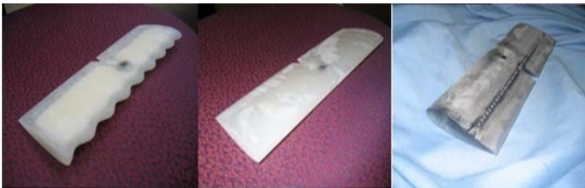
FIG 2.12 The full-span foils with tubercles (left), unmodified (middle) and the model with vortex generators (right) used by Stein et al. [112]
