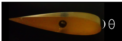
Figure 2. Side view of the wavy wing section, showing the peak-to-peak angular amplitude, \theta (deg)
