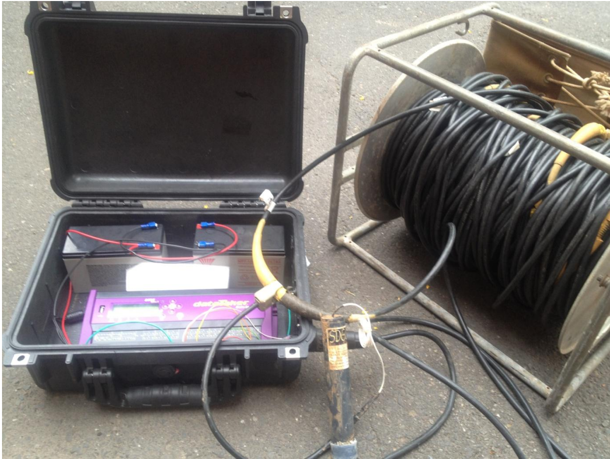
Figure 15: Photograph of prototype SP field logger model. The black casing (left) is a watertight hub (approximately 40 cm length) for non-water resistant logger controls. It contains the general purpose datalogger DataTaker DT8,5 where the logger program is commenced and halted. The datalogger also allows for live inspection of electrode values (in mV) to detect for electrode issues. Batteries are sealed within this box, and a solar panel is used to hold battery charge. Additional batteries can be plugged in externally via water tight connection. The adapted seismic cable (right) has a total length of 120 m, with yellow take-out measurement points for modified geophone connector electrodes (central). The electrode displayed is a SDEC France's PMC900, Pb-PbCl 2 NaCl unpolarizable electrode.
