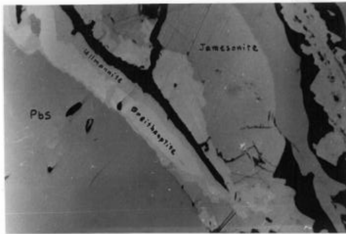
FIG. 27 Breithauptite and ullmannite. Note ragged boundary against galena and jamesonite. x 250
