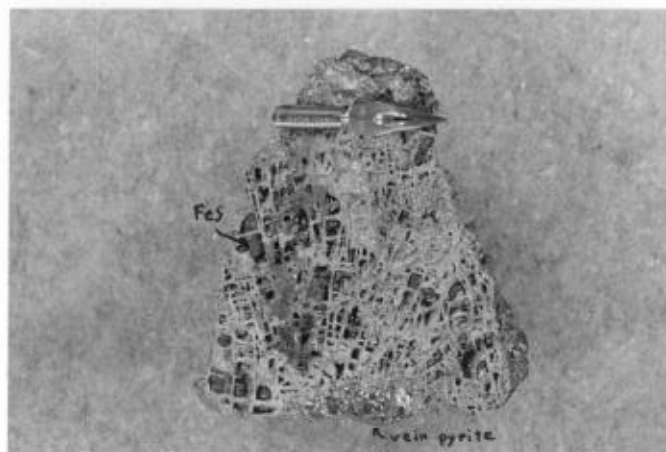
FIG. 9 Secondary \text{FeS}_2 boxwork containing remnants of \text{FeS} . Note shiny cube of unaltered vein pyrite. x \frac{1}{2}
