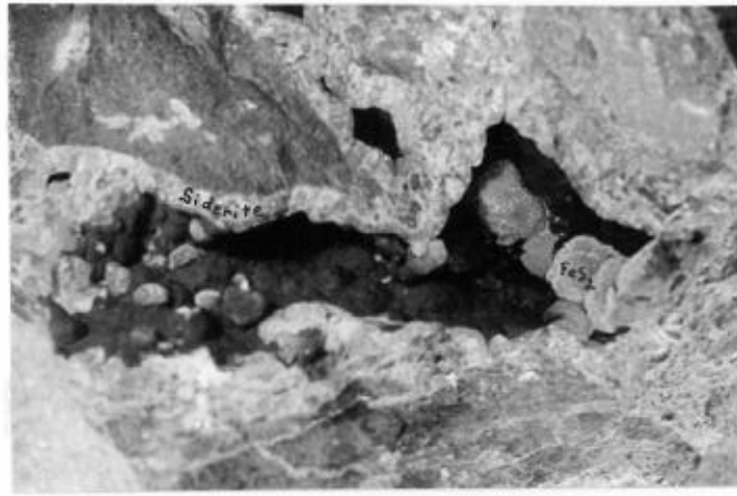
FIG. 13 Cavity containing patches of \text{FeS}_2 on limonite on siderite. \times 3/4
