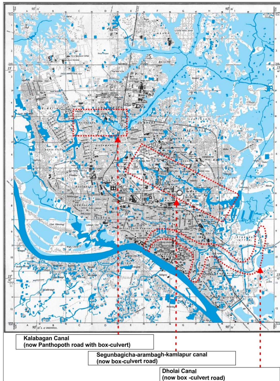
Figure 5-18: 1960 Map showing different water channels and wetlands including urbanised area. (source: Drawn by the author from the collected map from the Department of Architecture BUET, the original map was prepared by the Pakistan Government in 1960 based on the survey of 1959-60)
