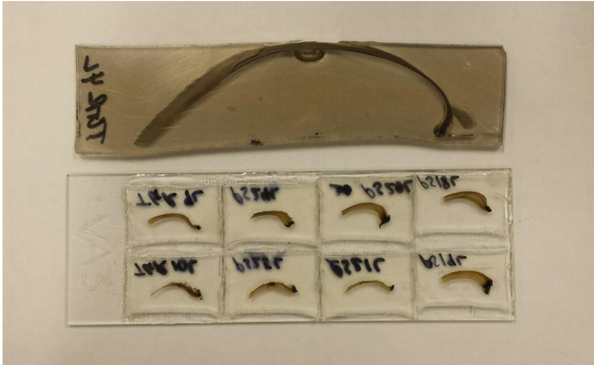
Figure 3: Full growth axis section (top - SEM analysis) and mounted umbo sections on glass microscope slide (bottom - LA-ICP-MS analysis).
