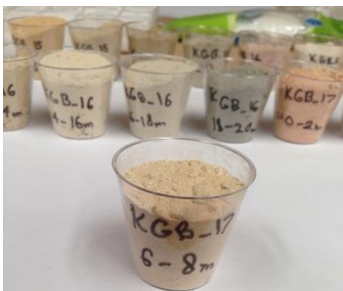
Figure 3: 30mL container of powdered rock, labelled with drill hole and depth, ready for transfer to pXRF plastic cup for analysis
