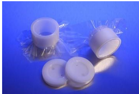
Figure 4: Assembled pXRF sample holder showing X-ray film base.
