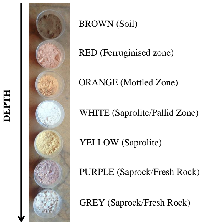
Figure 6: Crushed sample colour. The pattern Brown → Grey was often seen as holes increased in depth.
