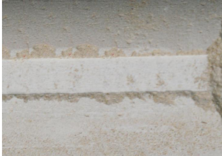
Fig. 4.15 Failure surface profile for Savonnières sample for \alpha=45^\circ and d = 1.3 mm.
