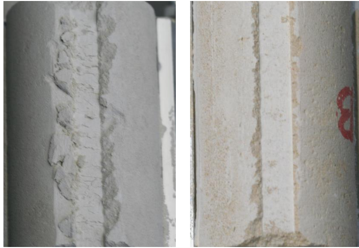
Fig. 4.17 Failure surface profile for Tuffeau sample (left) and Savonnières sample (right) at \alpha=45^\circ and d = 1.4 mm.
