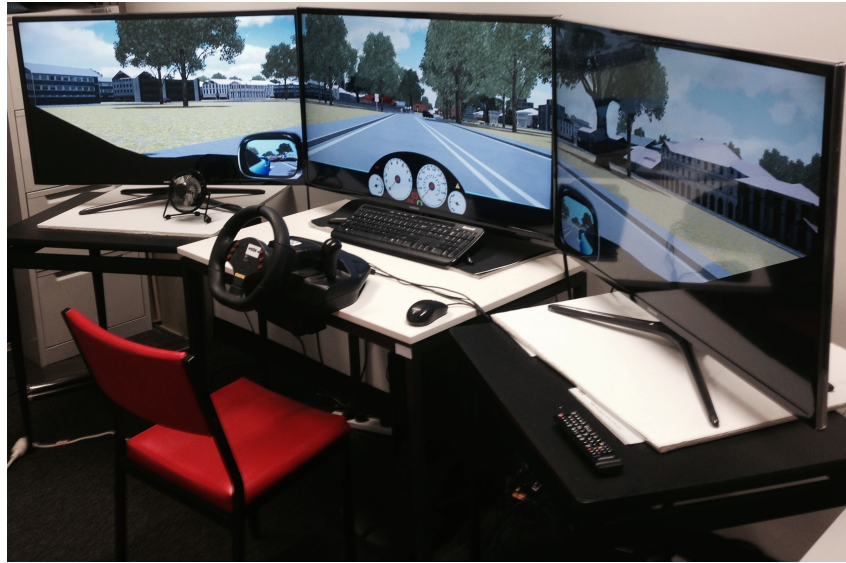
Figure 5.1: Driving simulator setup
