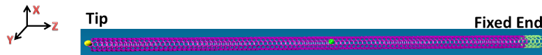
Figure 7.19: CNT atom positions used to observe the displacement of the tip and the middle of the CNT.
