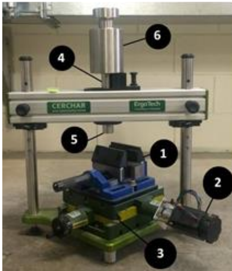
Figure 6-2. Modified Cerchar apparatus: 1-Sample holding vice, 2-Electric motor, 3-Two axis cross table, 4-Tool holder, 5-Pin and 6-Normal force.
