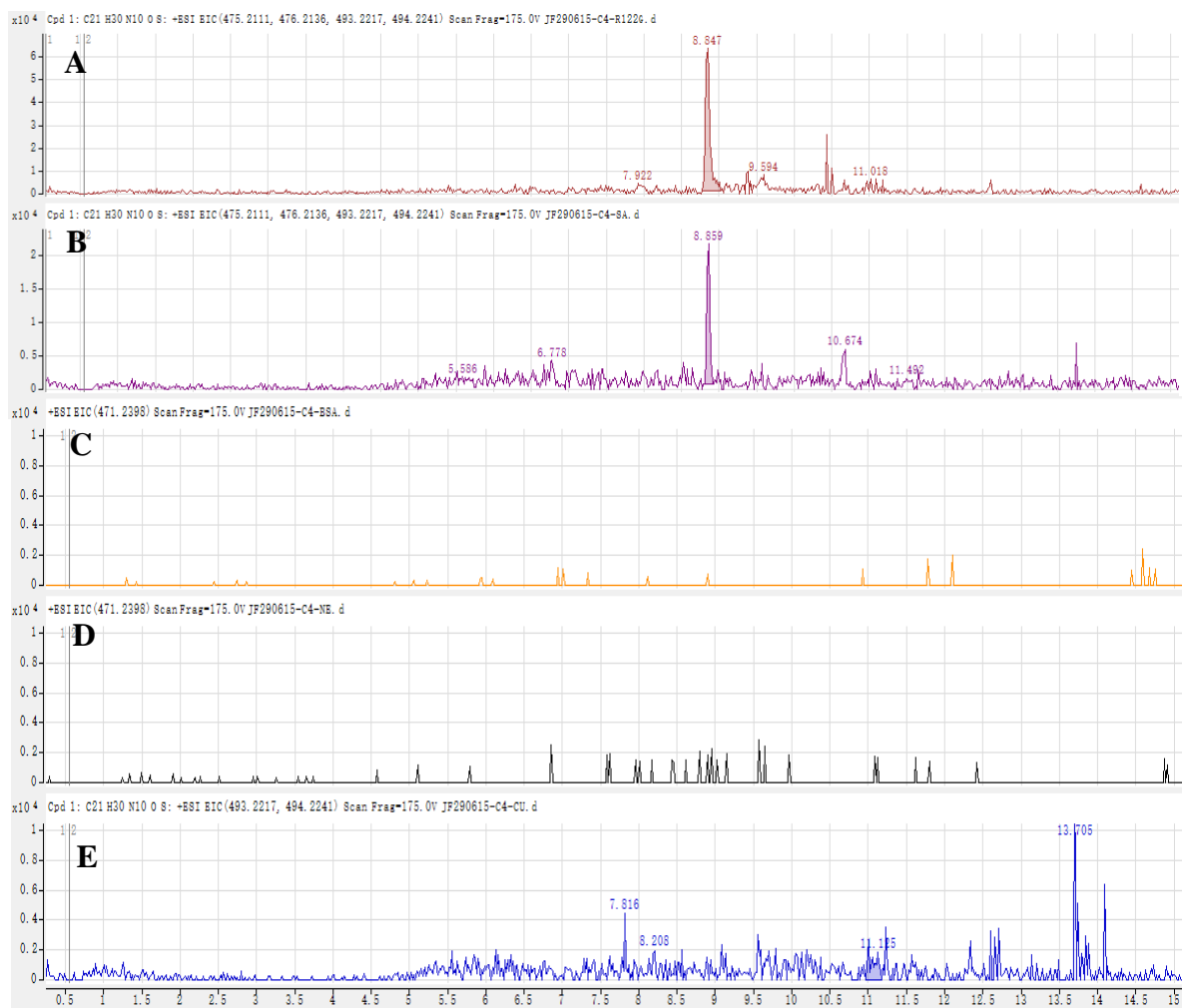
Figure 10: LC/HRMS traces of reference compounds and in situ click produced triazole 6.27 at selective ion monitoring ( \text{M}+\text{H}^+ = 471.2398 Da). (A) Product from in situ assembly in the presence of SaBPL . (B) Product from in situ assembly in the presence of SaBPL-R122G . (C) Control using BSA. (D) Controls (no enzyme). (E) Control using \text{Cu}_2\text{SO}_4 (5 \mu\text{M} ).
