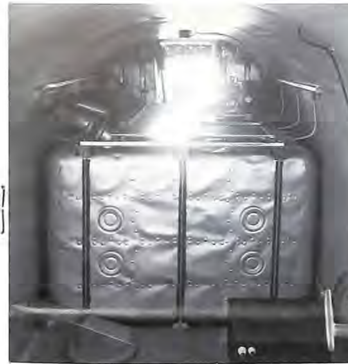
Main fuel tanks as installed in Earhart's Electra. Photo courtesy Lockheed Corp.
