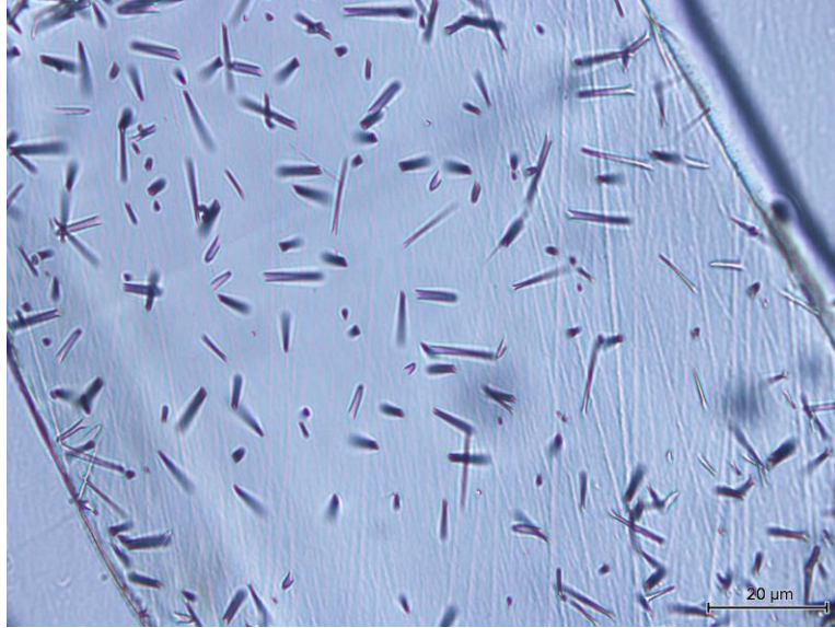
Figure 2: An example of an etched apatite grain with spontaneous fission tracks (dark lines within the crystal). The photo was taken using transmitted light on an Olympus BX51 Microscope, with an Olympus DP21 camera and computer attachment, on 1000x magnification.
