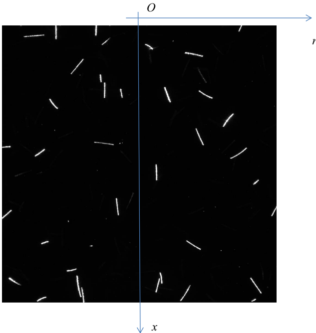
Fig. 4. A typical raw image obtained at the exit plane of the jet together with the coordinate system for the fibrous particles.
