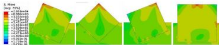
(c) Von-Mises stress distribution of the system having the square particle
