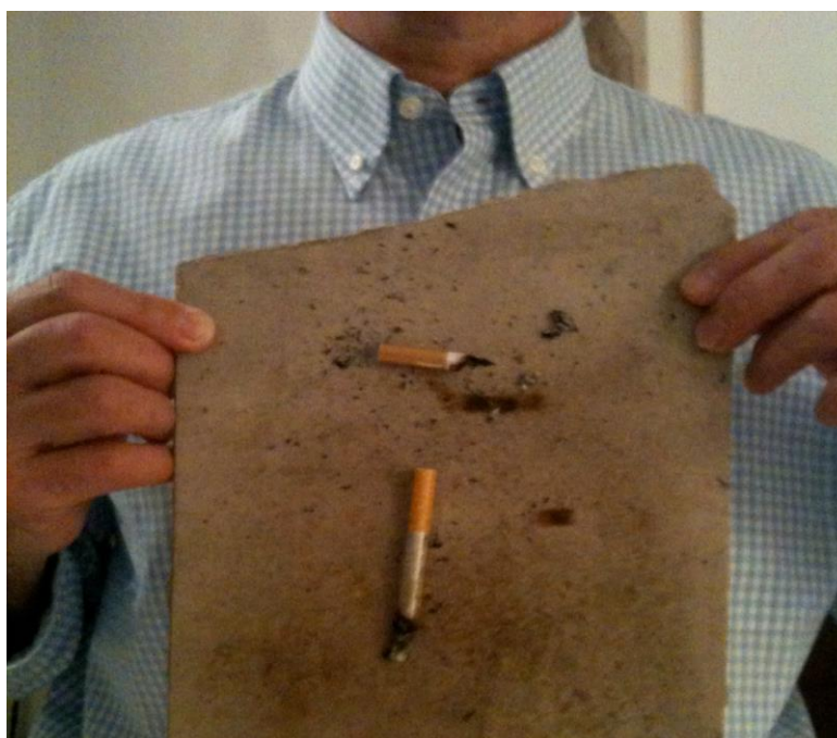
Figure 4. The bottom cigarette and its ash are seen remaining in situ when sprayed with the tile turned up.
