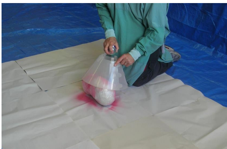
Figure 5. Stone model of a head sprayed with containment device allowing measurement of aerosol radius.
