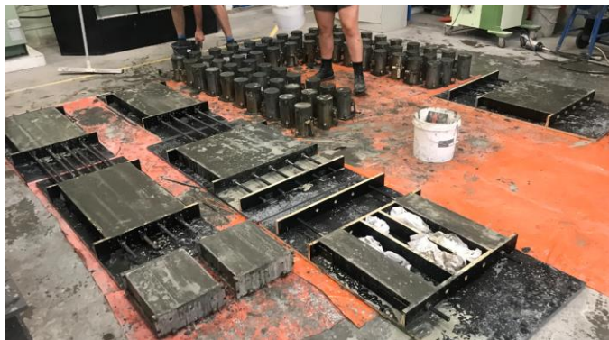
Fig. 3.4 Immediately after pouring concrete mix in to the moulds for different test specimens.
