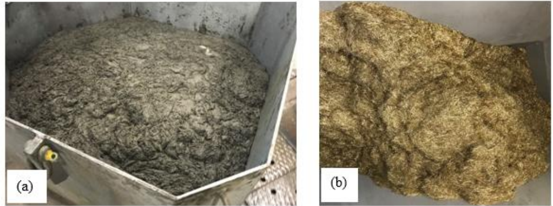
Fig. 3.2 (a) Fresh concrete mix of UHPFRC at laboratory and (b) picture of steel fibers.
