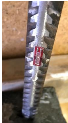
Fig. 3.8 Electronic strain gauges on reinforcement.
