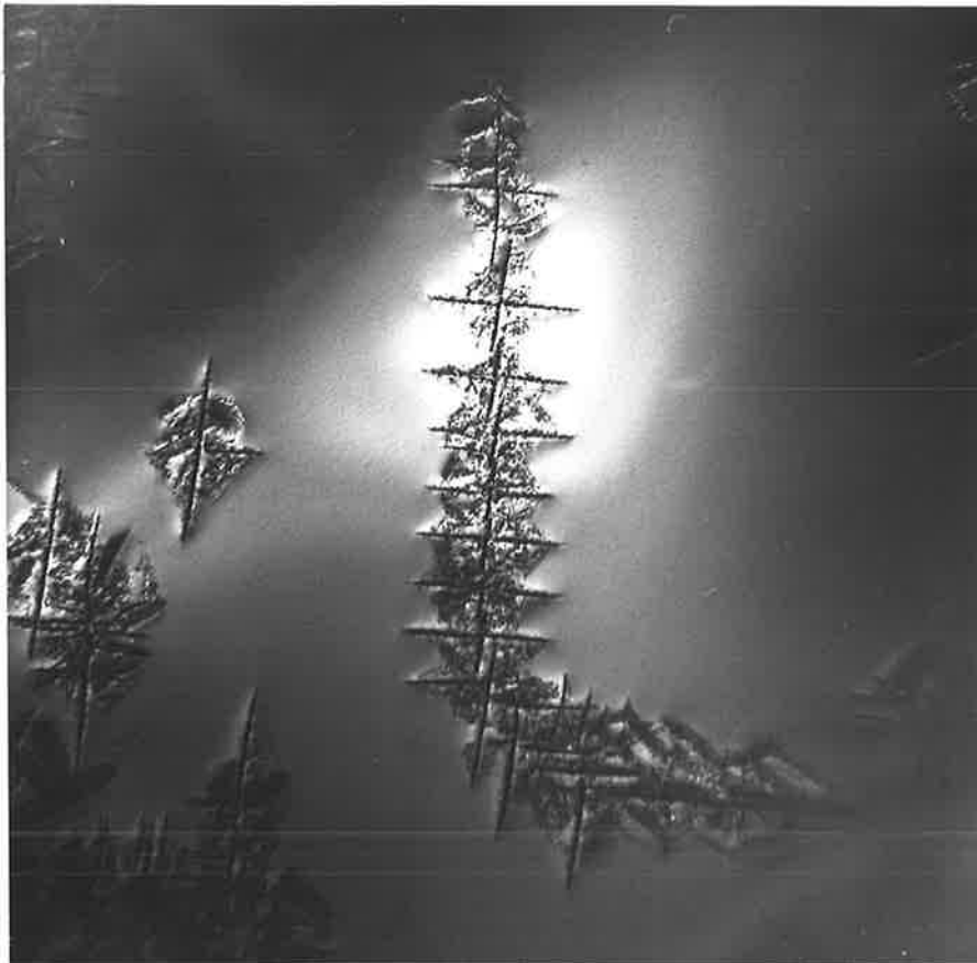
Fig. 4.8 Fe-13Mn-7Mo-0.8C aged at 750°C for 1 hour. Thin foil electron micrograph x 13,000
