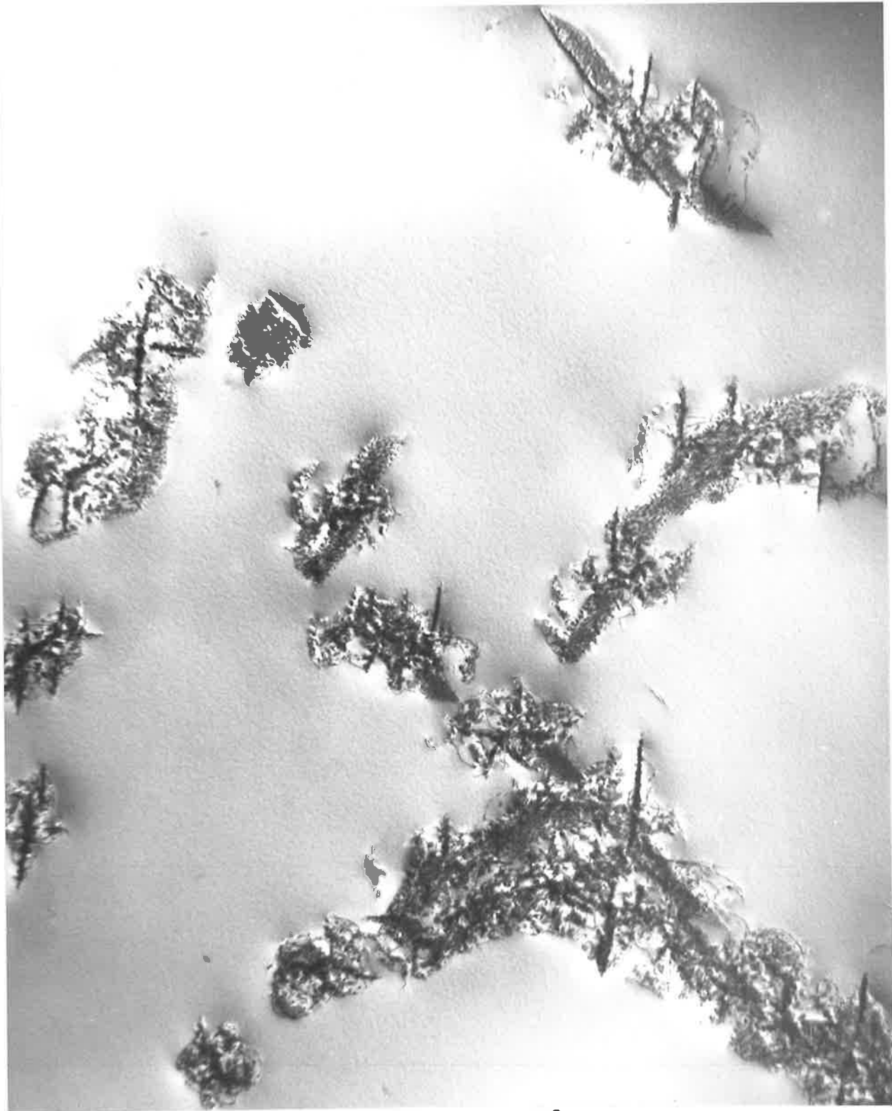
Fig. 4.6. Fe-13Mn-7Mo-0.8C aged at 750°C for 1 hour. Thin foil electron micrograph x 21,000
