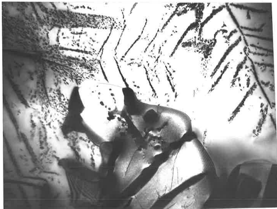
Fig. 4.16 Fe-13Mn-4Mo-1.2C aged at 750°C for 5 hours. Thin foil electron micrograph x 14,000
