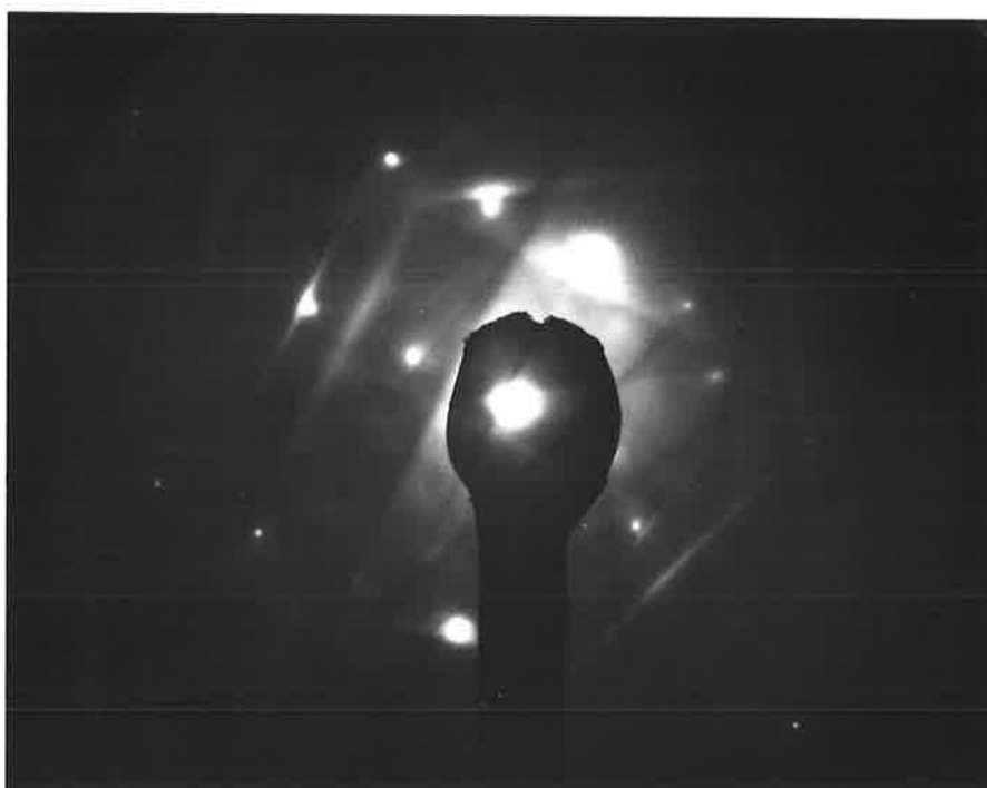
Fig. 3.5b. [31\bar{24}92] Kikuchi pole of the adjacent austenite.
