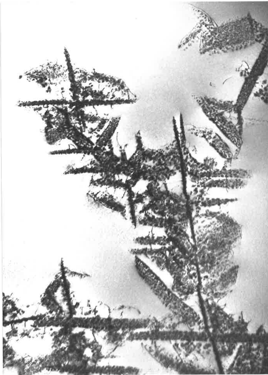
Fig. 4.3. Fe-13Mn-7Mo-0.8C aged at 750°C for 1 hour. Thin foil electron micrograph x 25,000
