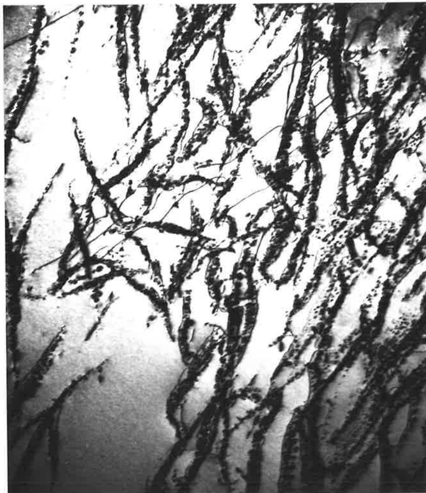
Fig. 4.11 Fe-13Mn-7Mo-0.8C deformed 5% and aged at 750° for 1 hour. Thin foil electron micrograph x 15,000
