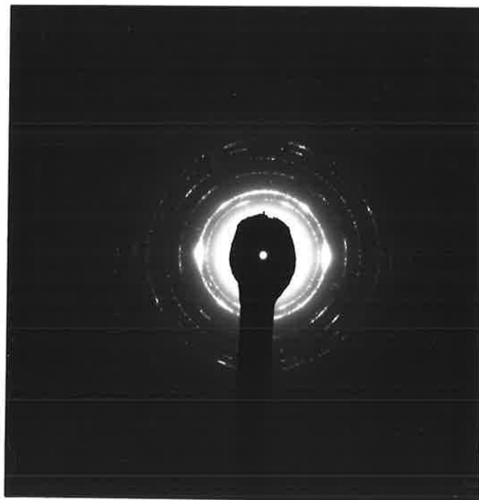
Fig. 4.4b. SAD ring pattern of fine precipitates in fig. 4.4a.
