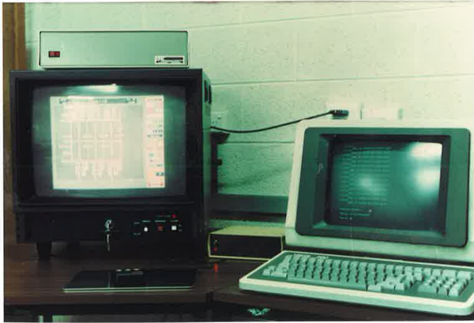
Figure 2.2 (c): Another colour graphics workstation, a VECTRIX [37] with optical mouse for cross hair control. Note also the monochrome terminal alongside used for displaying additional menus and allowing the use of a text editor, or alternatively some other CAD Tool while viewing the circuit on the colour monitor. Also compare the bulky bitpad in (a) with the much more compact optical mouse shown here.
