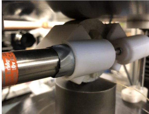
Figure 3.14: Smooth contact between disc sample and loading plate
