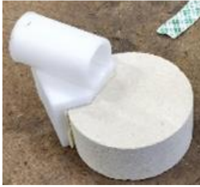
Figure 3.12: Specimen and holder bonding
