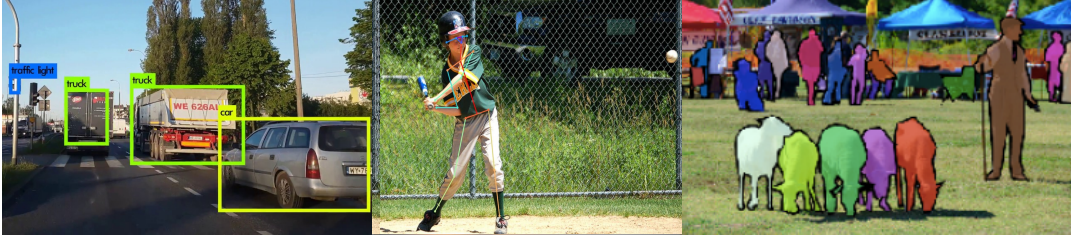
FIGURE 1.1. Instance-level recognition tasks. From left to right: object detection; keypoint detection; and instance segmentation.
