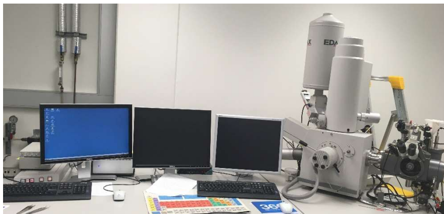
Figure 2. 7. The Philips XL 30 Field emission scanning electron microscope at Adelaide Microscopy Centre.
