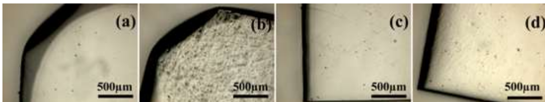
Figure 7. 14. IM128 glass surface images (cladding glass): (a) before annealing at 322 °C for 10 hours; (b) after annealing at 322 °C for 10 hours; (c) before annealing at 318 °C for 10 hours; (d) after annealing at 318 °C for 10 hours.
