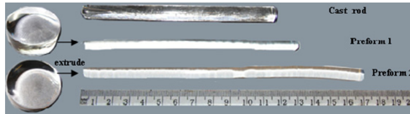
Fig. 1. Fluoroindate glass in the form of: (Left) Cast billets. (Top) Cast rod. (Centre) Preforms cast from cast billets.
