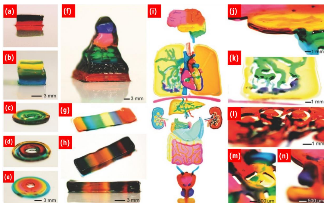
Figure 2.4. 3D bioprinted architectures through swift continuous multi-material extrusion-based bioprinting. (a) Dual-layered cuboid block, (b) triple-layered cuboid block, (c-e) blood-vessel like constructs of dual, triple, and quadruple materials, respectively, (f) seven material-containing pyramid, (g-h) continuous segments of seven different bioinks in three- and ten-layered blocks, (i) separately printed organ-like constructs from multiple bioinks, (j-n) side views of constructs in ('i') to show 3D nature; (j) brain, (k) lung vascular, (l) kidney, (m) left atrium (heart), (n) bladder/prostate [24] . Reproduced with permission from ref. [24] , Copyright (2016) Wiley-VCH.
