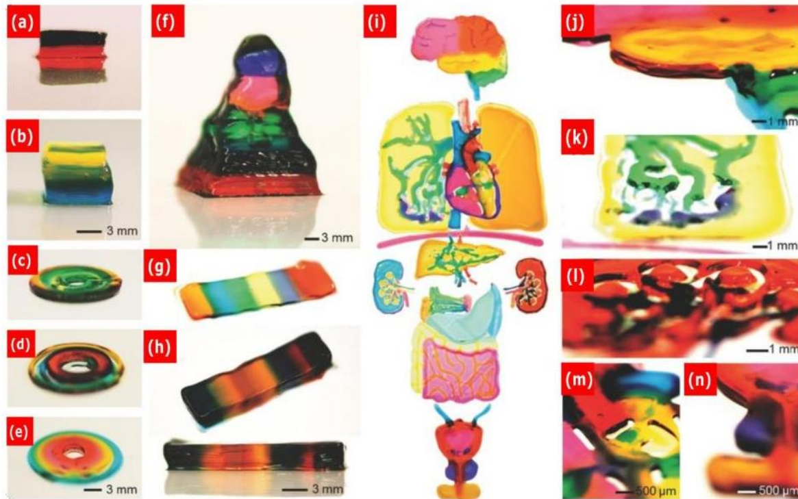
Figure 4. 3D bioprinted architectures through swift continuous multi-material extrusion-based bioprinting [49]. (a) Dual-layered cuboid block, (b) triple-layered cuboid block, (c-e) blood-vessel like constructs of dual, triple, and quadruple materials, respectively, (f) seven material-containing pyramid, (g-h) continuous segments of seven different bioinks in three- and ten-layered blocks, (i) separately printed organ-like constructs from multiple bioinks, (j-n) side views of constructs in ('i') to show 3D nature; (j) brain, (k) lung vascular, (l) kidney, (m) left atrium (heart), (n) bladder/prostate. Reproduced with permission from ref. [49], Copyright (2016) Wiley-VCH.
