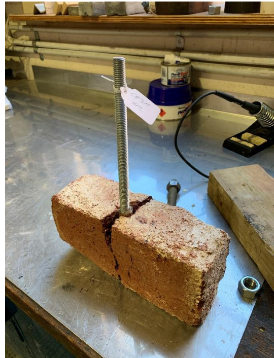
Fig. 24 – Anchor failure under impact loading – new brick
