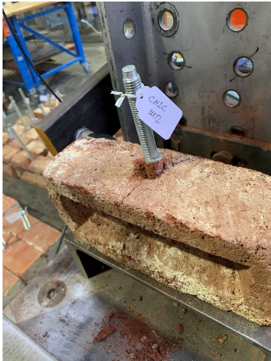
Fig. 23 – Anchor failure under cyclic loading – new brick
