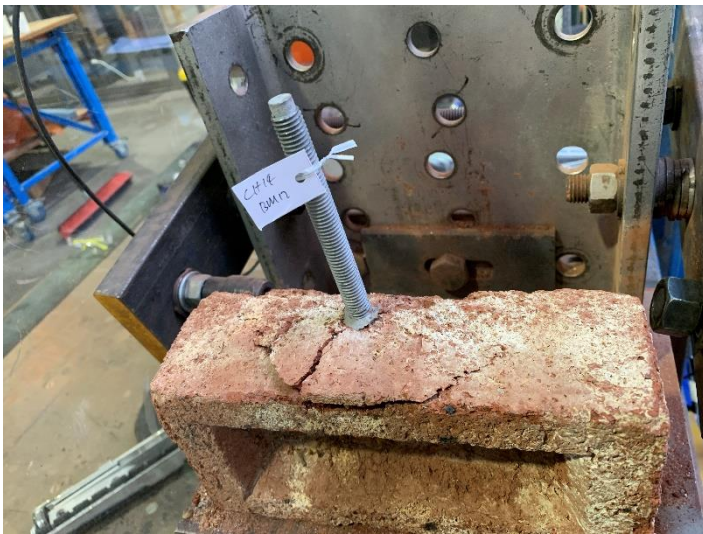
(a) short hole (note localised cone failure)
