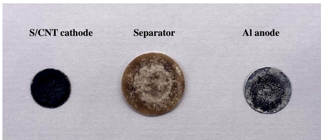
Supplementary Figure S15 Digital photos of sulfur cathode, separator and Al anode disassembled from the cycled Al-S batteries.
