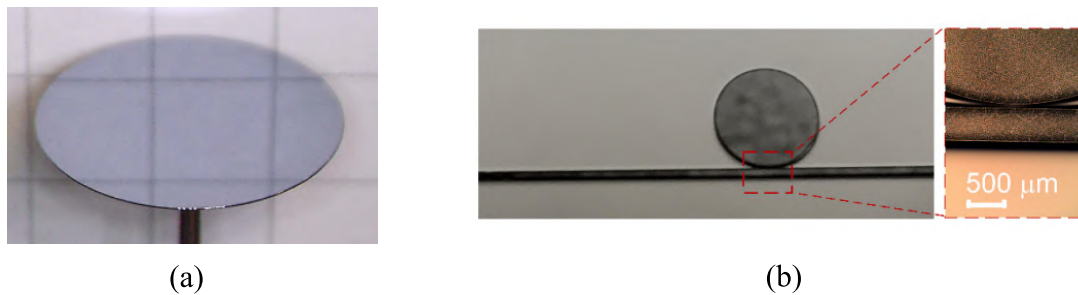
Figure 1.9. Existing disk resonators. (a) Silicon disc microresonators. Adopted from Vogt et al. (2020), and (b) Disk cavity. Adopted from Xie et al. (2018).
