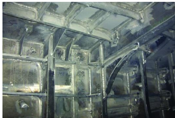
Fig. 1.1. T-welded joints in ship hull structures [6]
