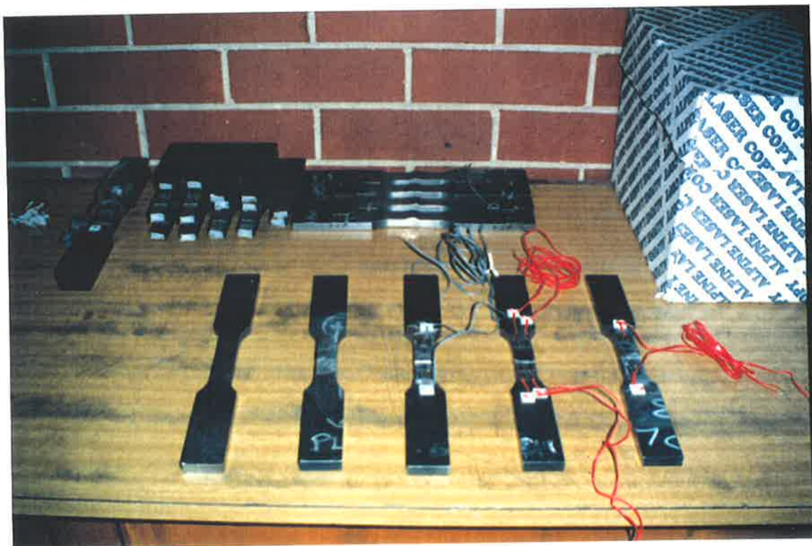
Figure 4.4 Test specimens with strain gauges bonded at the weld toes
