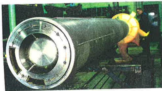
Figure 1.2: A 100 MW Gyro-Therm burner for a cement kiln in Geelong, Australia
