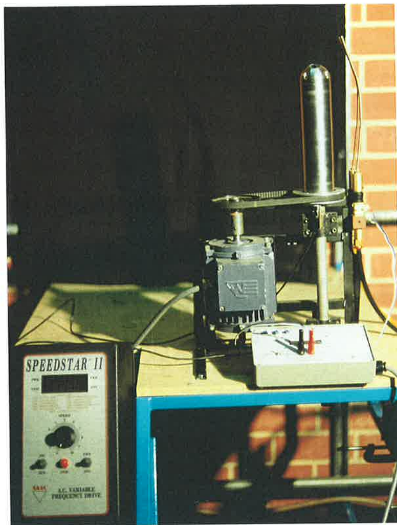
Figure 2.13: The smoke visualisation system mounted beside the nozzle and its variable speed drive. \text{NH}_3 and \text{SO}_2 are pulsed through two thin tubes to the right of the nozzle
