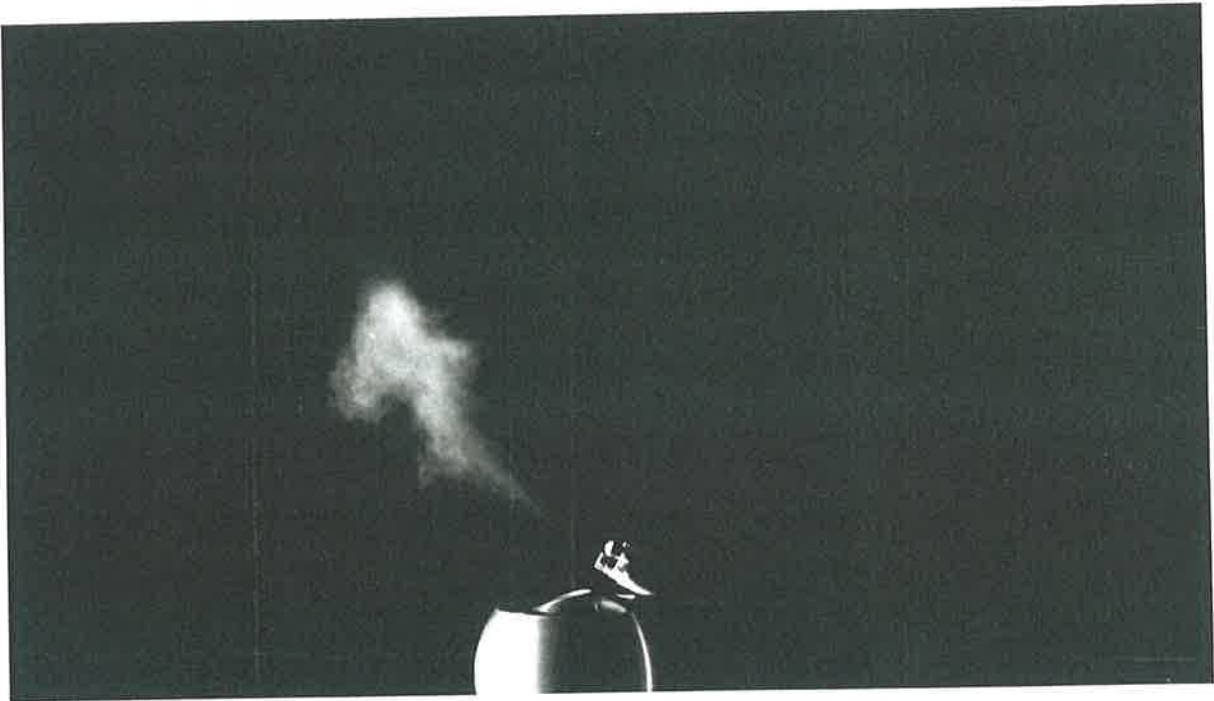
Figure A.1: Conditional smoke visualisation. St_p=0.002 , Re=26,600 .
