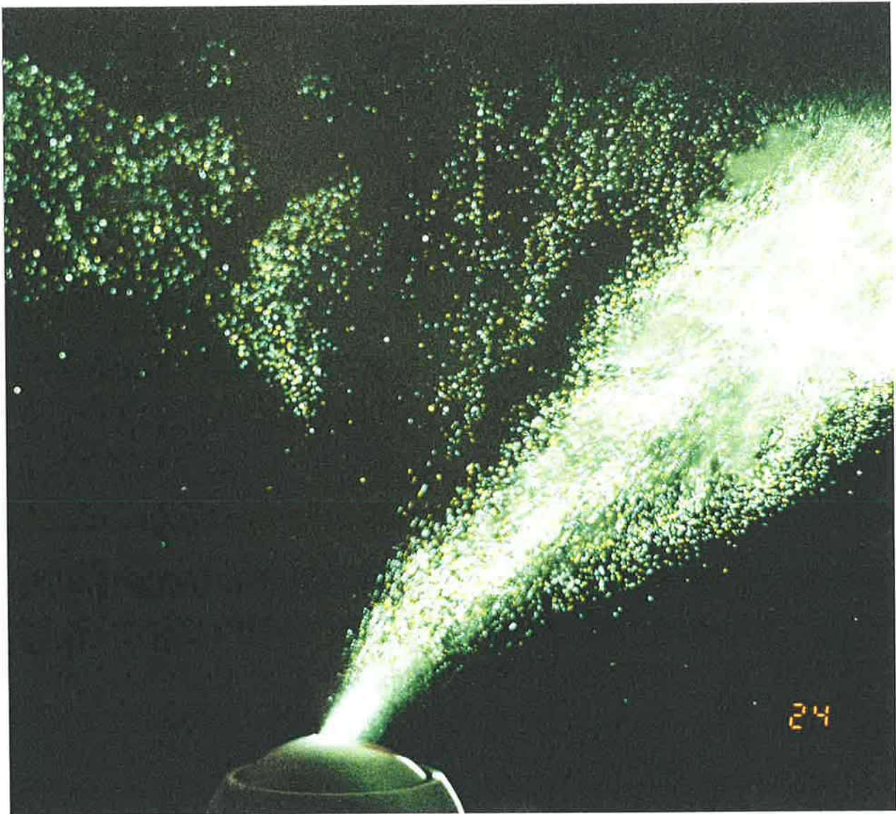
Figure 3.12: Vertical Light Sheet from 0 < x/d_e < 12 through the r-x Plane in the low Strouhal number Jet marked with glass beads. St_p = 0.002 .
