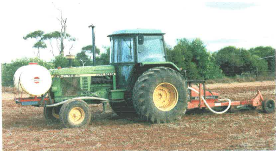
Plate 3.1 Equipment used in the field experiments to inject nutrients into the subsoil to a depth of 0.40 m.
