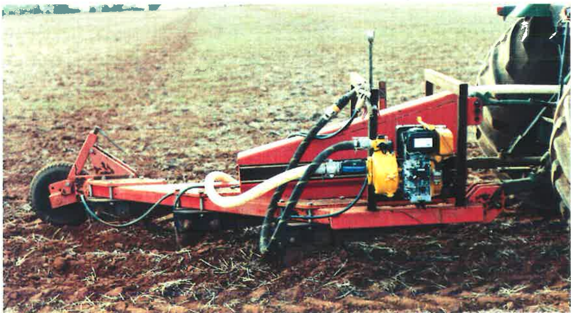
Plate 3.2 The Howard "Paraplow" used in the field experiments to inject nutrients into the subsoil to a depth of 0.40 m.
