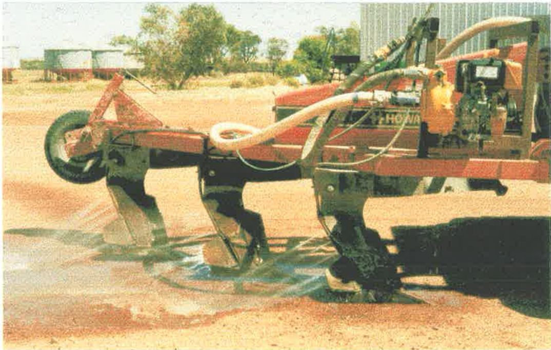
Plate 3.3. Method of delivery of nutrients to the subsoil.
