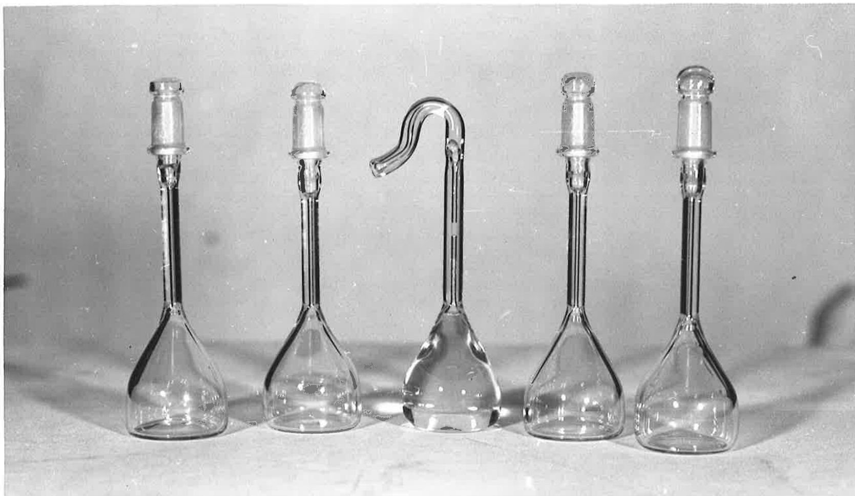
Plate 4.1. The four pycnometers and tare used for density measurements in this work.
