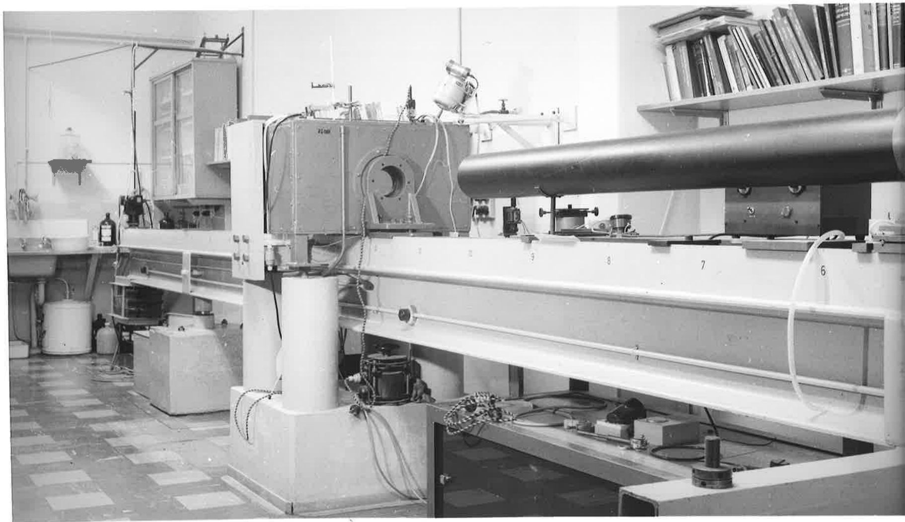
Plate 5.2. The Gouy diffusiometer.
