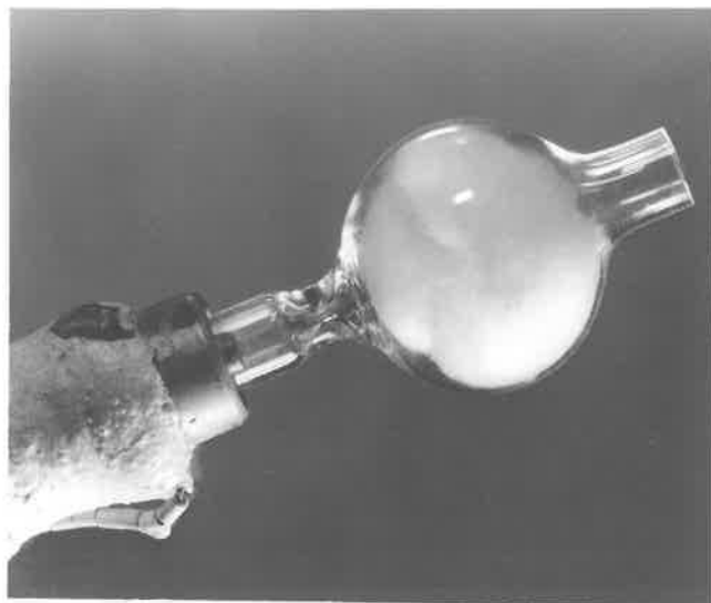
Fig. 5 Apparatus used for collecting the eluant vapour containing ^{14}\text{C} labelled fatty acids after gas liquid chromatography. The calcium chloride tube is fitted into the outlet tube by means of a silicone rubber joint.
