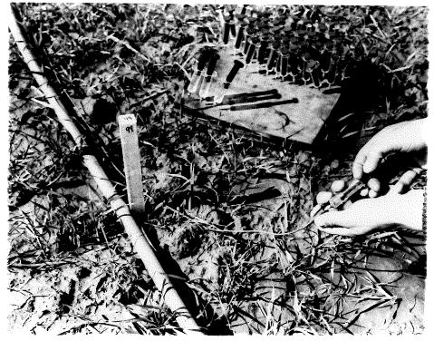
The reservoirs were placed on a thin (1 cm) bed of fine washed building sand at the bottom of a 6.1 cm diameter hole, made with a Stace-Palm modified Veihmeyer tube (Stace and Palm, 1962). Sand was used to pack the gap between the walls of the can and those of the hole. The soil was replaced with frequent tamping. Fig. 1a is a diagrammatic representation of these operations, and Fig. 2 is a photograph of one of the installed reservoirs.
