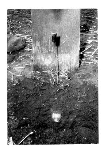
Figure 2. Soil gas reservoir at the 15 cm depth, partially excavated after the conclusion of Experiment I.
