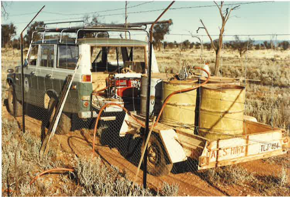
Fig 4.1a The equipment used to transport and pump water to the irrigation plots. In the foreground is the kangaroo-proof fence.
