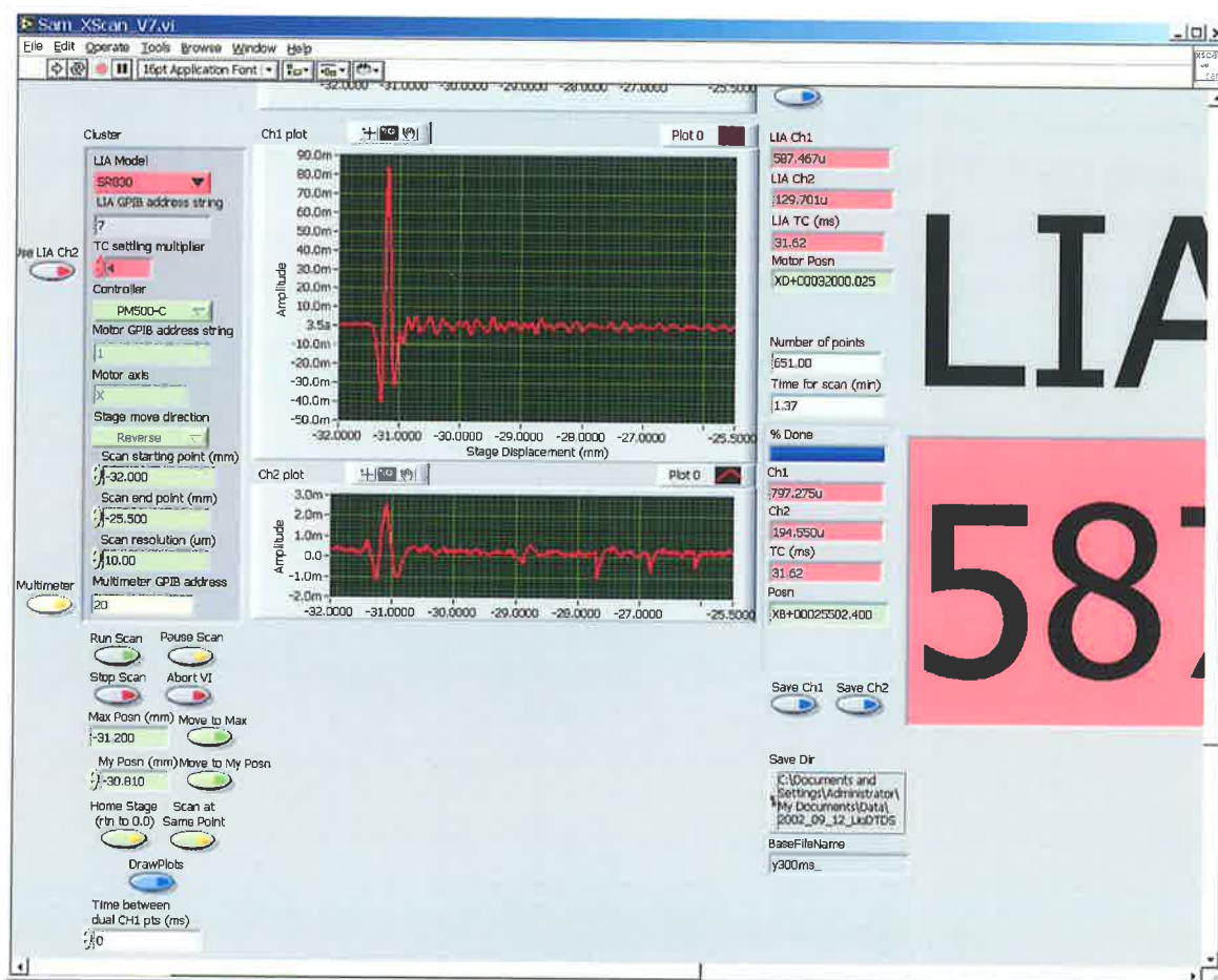
Figure B.5. Screen shot of control software for operating T-ray TDS experiments. This is a screen shot of the LABVIEW computer interface used to control the T-ray spectrometer used in this Thesis. The controls for the experiment are shown on the left and the readouts are on the right. In the centre is a large time-domain graph of a sampled T-ray waveform – the X-axis is a readout of the delay stage position and the Y-axis is channel one of the Lock-In Amplifier (LIAs). The smaller graph underneath shows channel two of the LIA, which should be much smaller than channel one if channel one is in phase with the optical modulator (chopper). The large display half-visible on the right-hand side was used for reading the LIA output from across the room when aligning certain optics.
