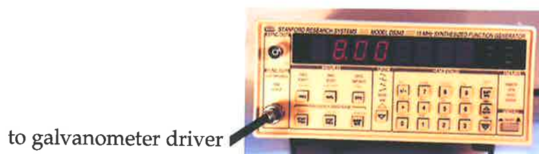
Figure 6.9. Photograph of a function generator used for double-modulated DTDS experiments. A Stanford Research Systems DS340 function generator was set to generate a sinusoidal 8.0 V peak-peak amplitude, which drove the DTDS galvanometer at 1 cm peak-to-peak.
