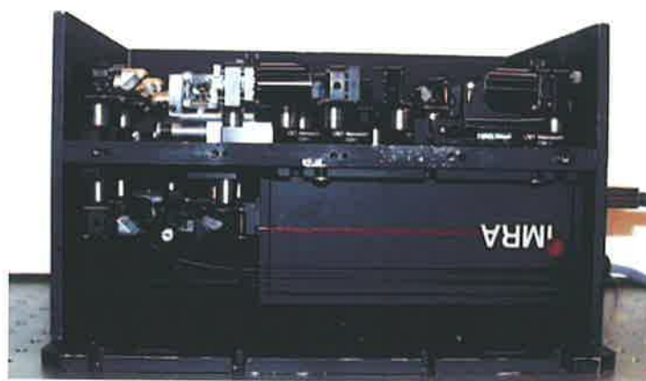
Figure 11.6. Compact T-ray spectrometer. This photograph shows a compact T-ray system, based on a fibre laser (manufacturer: IMRA America Inc., Ann Arbor, Michigan, USA; URL: http://www.imra.com ), sitting on a table with one-inch spaced holes (after (Li et al., 1999b)).
