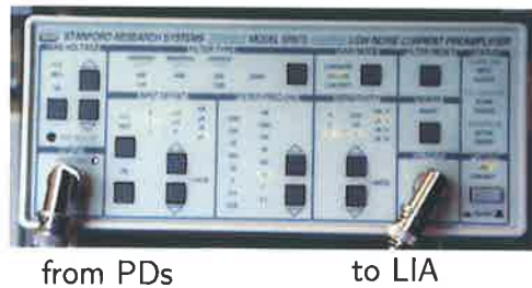
Figure B.10. Photograph of the low-noise current amplifier. Stanford Research Systems low-noise current preamplifier. The preamplifier took the current signal from the balanced photodetectors (PDs) and converted it to a voltage signal for the Lock-In Amplifier (LIA, see Sec. B.7.1). The main benefit of using the preamplifier was its adjustable gain-bandwidth product – the gain could be set sufficiently high to avoid any contributions from electronic noise without reducing the bandwidth below the modulation frequency (for example, the chopper frequency).
