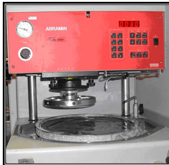
Figure 49: Abramin polishing machine (Struers, Copenhagen Denmark)
