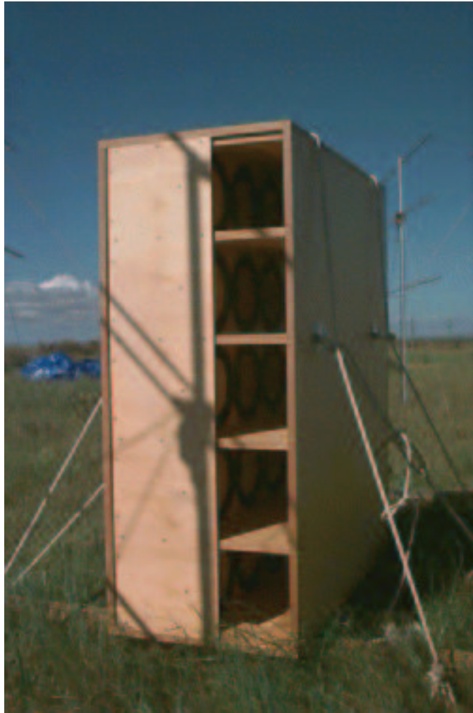
Figure 7.9: VAF E-115 RASS speaker at Buckland Park
