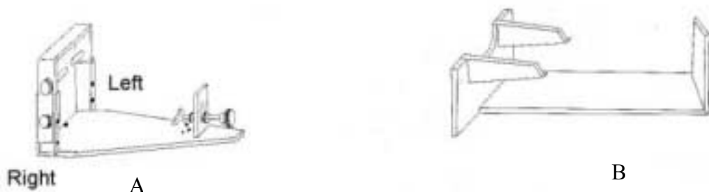
Figure 2.4. Cephalostat designed for sheep. A: Head frame with metal markers assisting calibration. B: Holder to stabilise the sheep head and the head frame.
