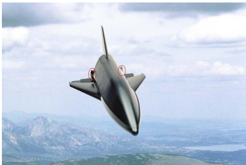
Figure C.1: The Hopper vehicle with speed brakes
