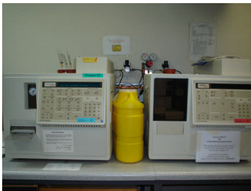
Figure 2.5 Gas chromatography system (Varian Australia): GC 3400 for measuring CO_2 concentration (left) and GC 3300 for C_2H_4 concentration (right)
