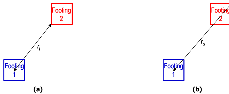
Figure 3-22 Determination of (a) internal and (b) external radius of annulus
