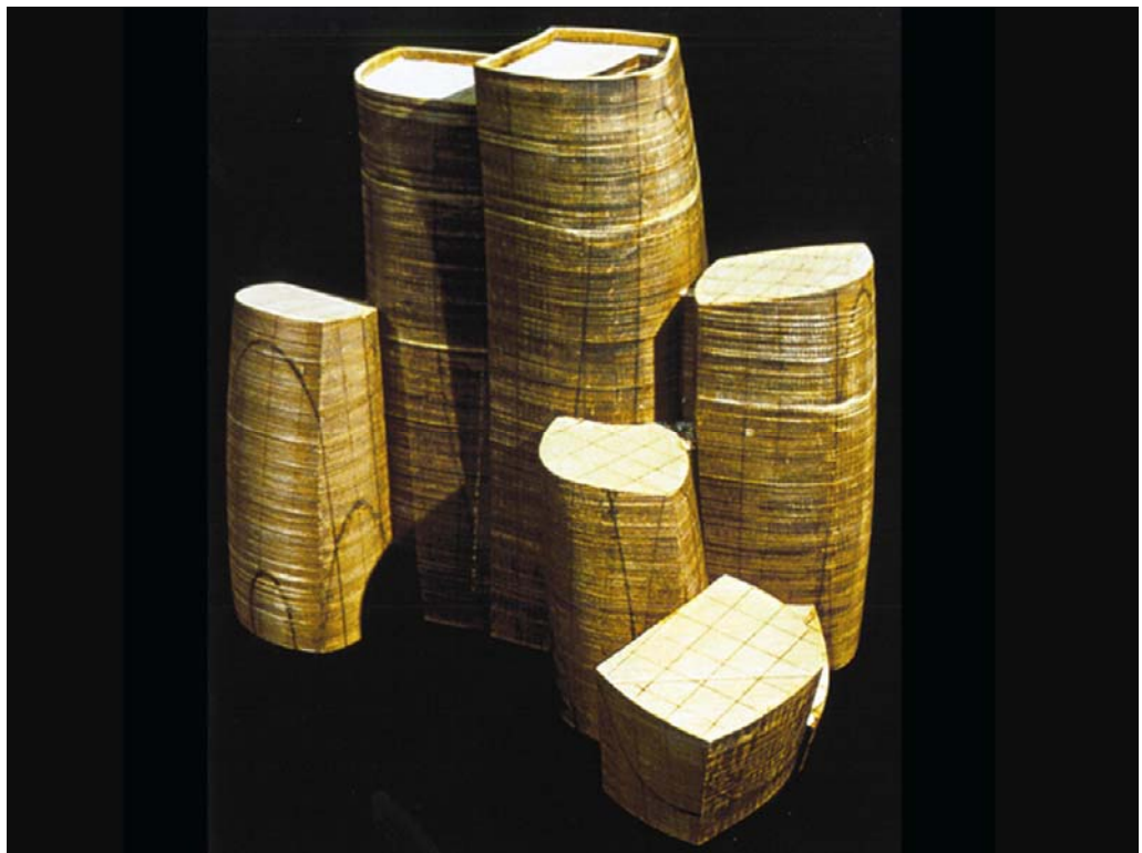
Figure 55 Laminated Object Manufacture Model, Der Neue Zollhoff.
