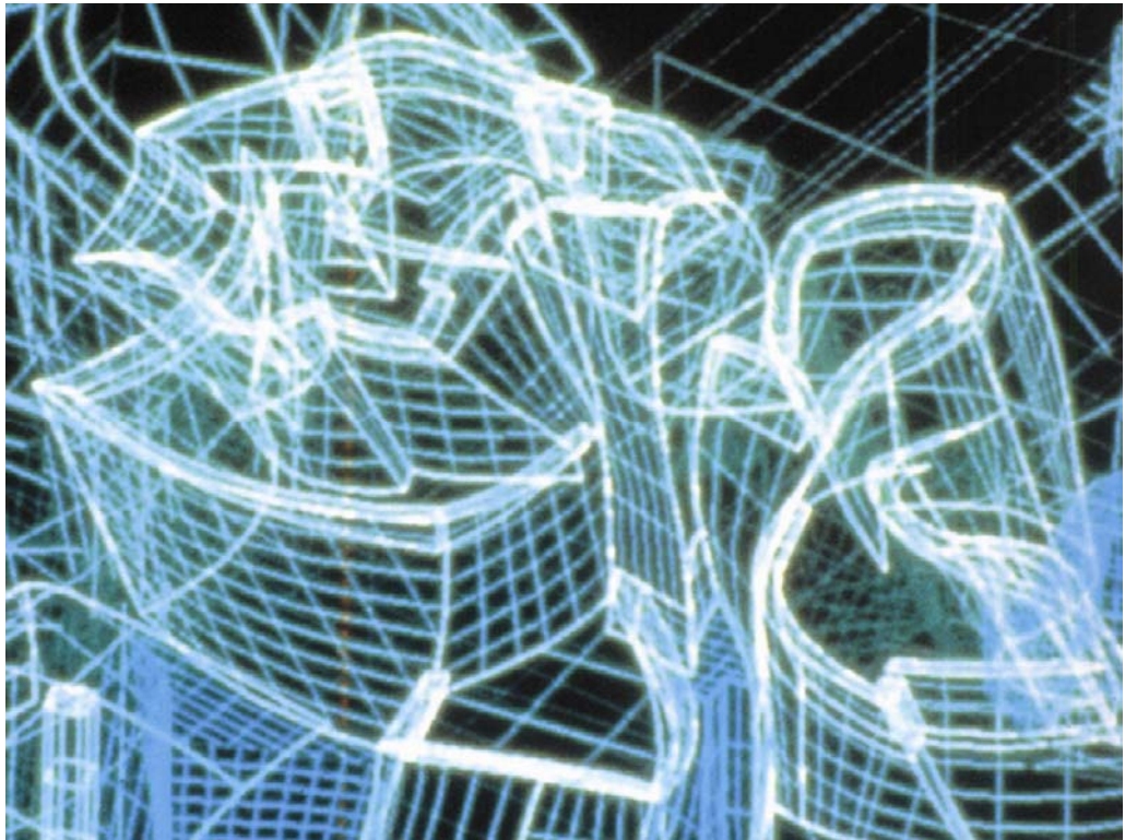
Figure 39 GMB, CATIA Wire Frame.
