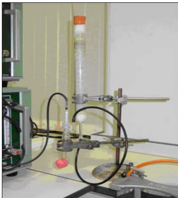
Figure 2-2 Purpose-made \text{CO}_2 scrubbing inlet carrier tube attached to IRGA for analysis of \text{CO}_2 in headspace from Exetainers.
