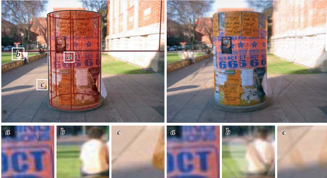
(a) The wire-frame projection of the hypothesised (b) Re-projection of all reference images back-surface super-imposed with the reference image. projected onto the surface.
