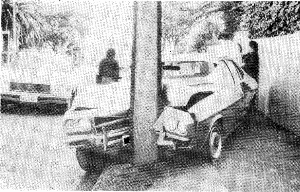
FIGURE 5.14: Subsequent collision with utility pole (Accident 090).
