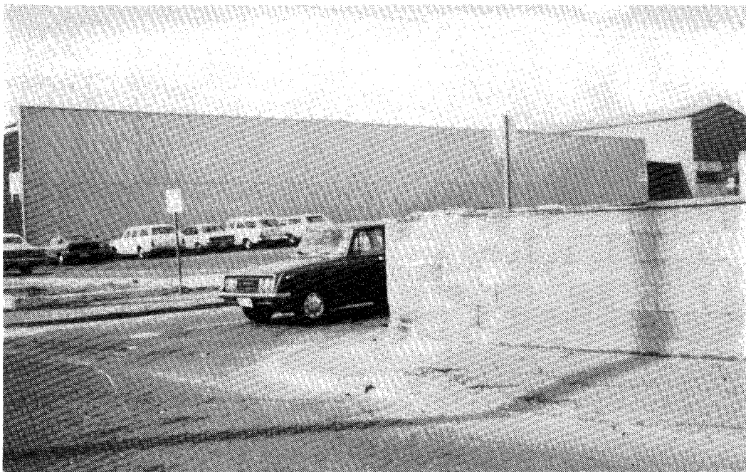
FIGURE 5.7: Severely restricted sight distance in Accident 017.
