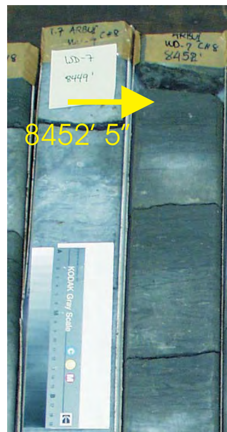
Figure 24A: Core Plug/Chip Atlas for sample 8452' 5" from Wiriagar Deep-7.
