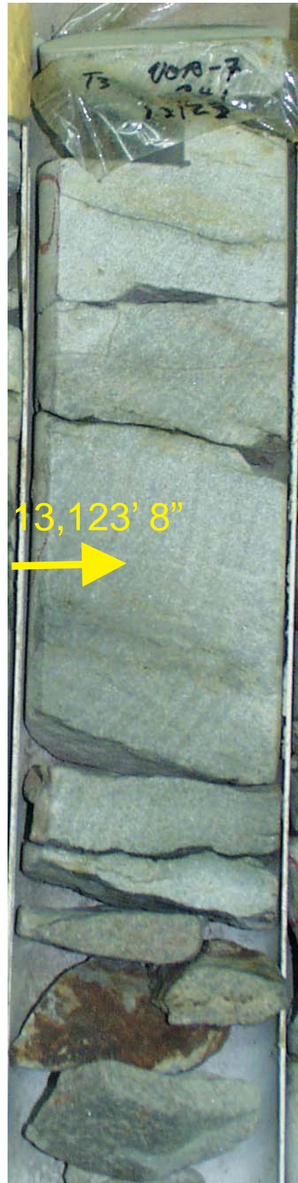
Figure 48A: Core Plug/Chip Atlas for sample 13123' 8" from Vorwata-7.
