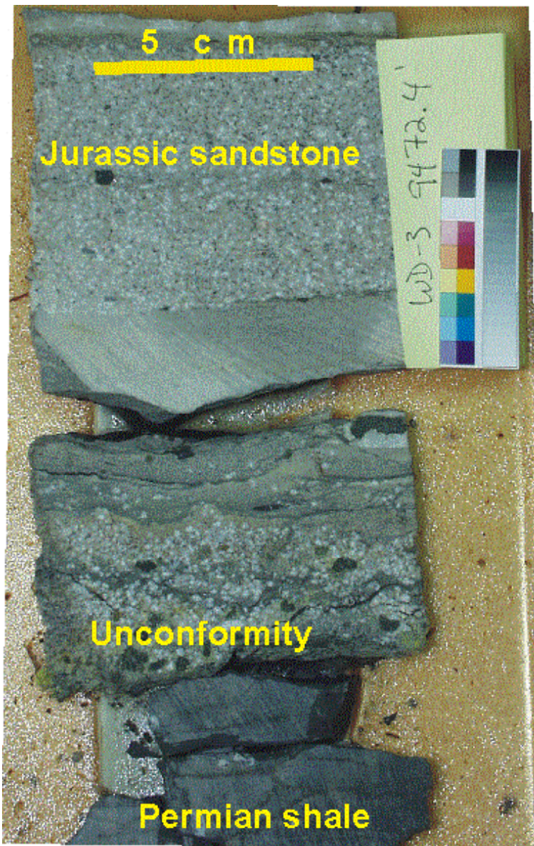
Figure 5.7: The Late Permian/Middle Jurassic nonconformable contact in WD-3 well, from Core No.15 at 9472 ft (driller's measured depth). Pebble lag at the base of the Jurassic is clearly visible.
