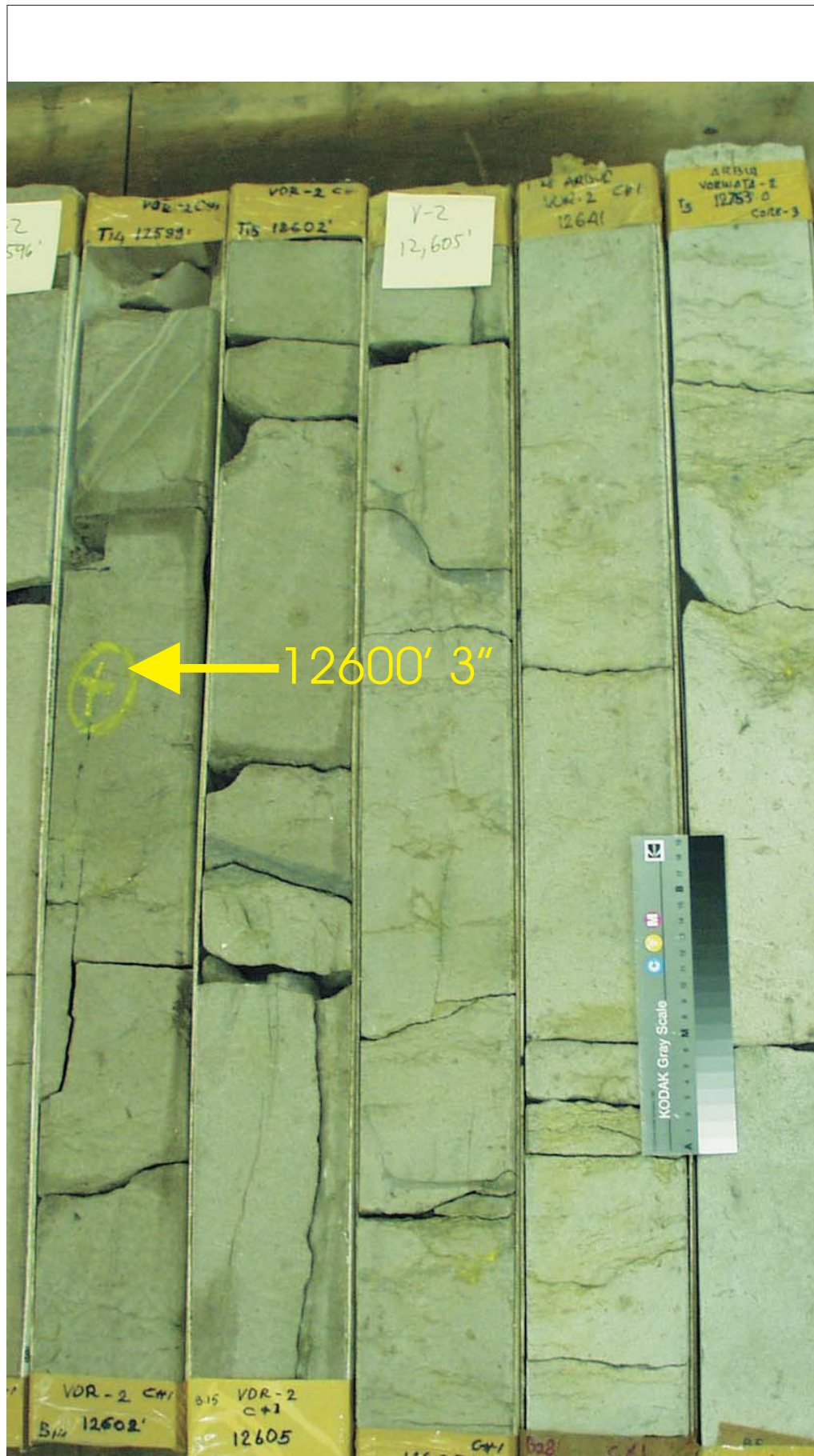
Figure 40B: Core Plug/Chip Atlas for sample 12600' 3" from Vorwata-2.
