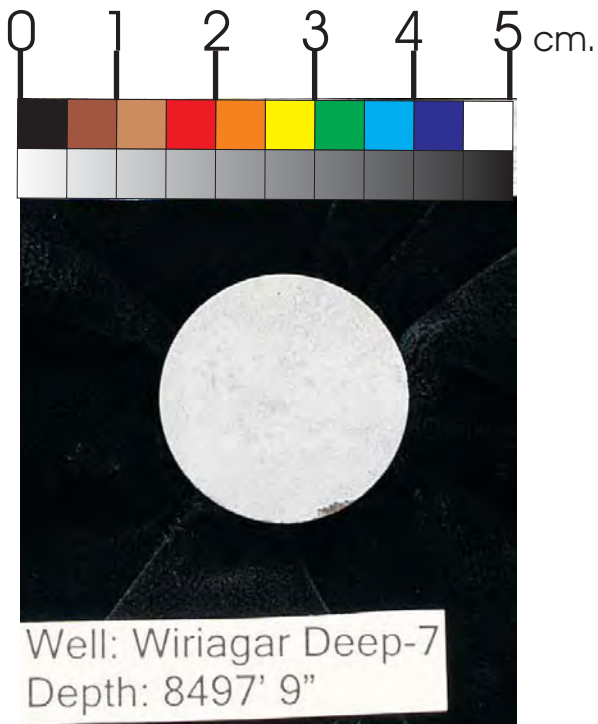
Figure 26B: Core Plug/Chip Atlas for sample 8497' 9" from Wiriagar Deep-7.
