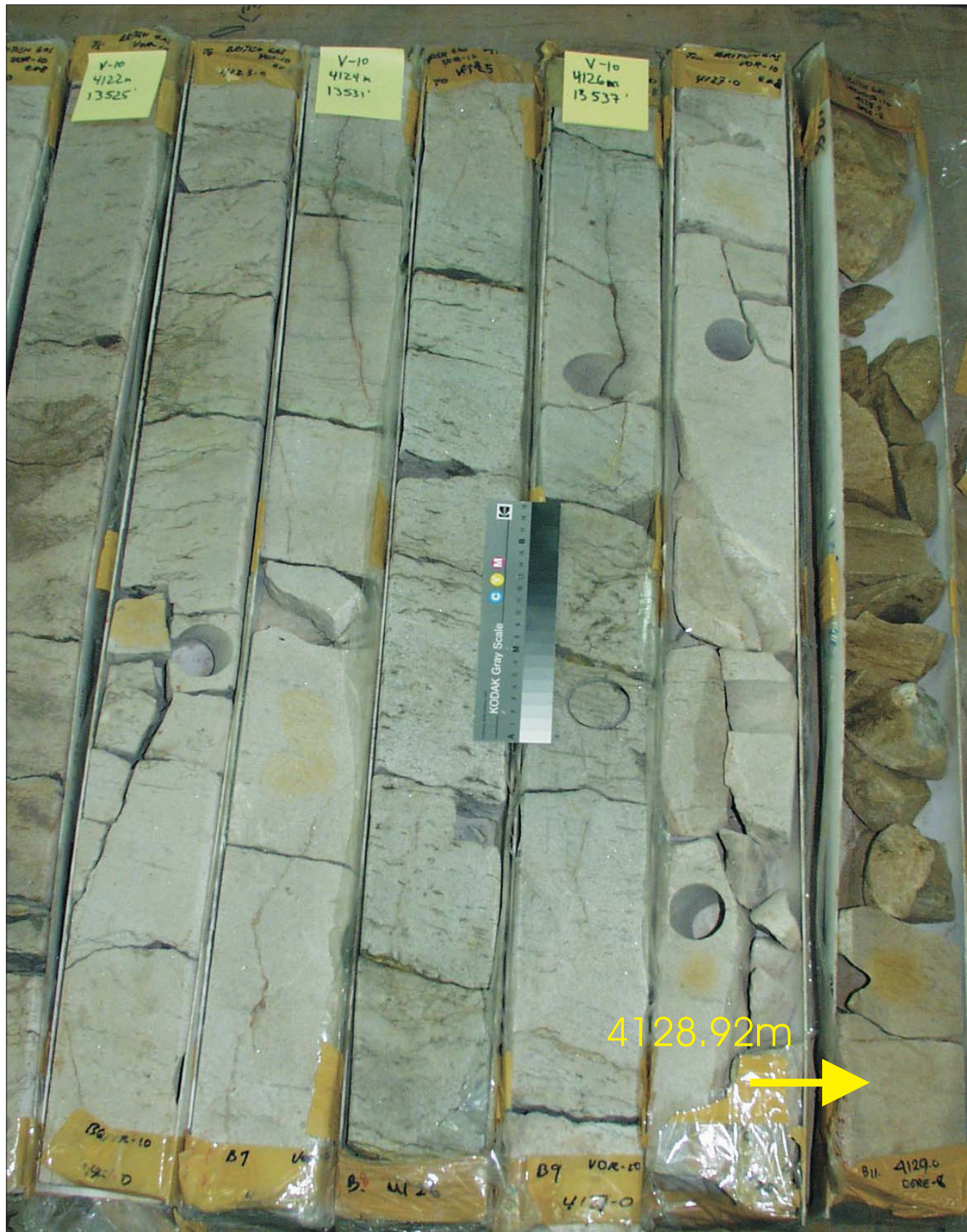
Figure 98A: Core Plug/Chip Atlas showing photographs and analyses results from sample depth 4128.92m from the Vorwata-10 well.
