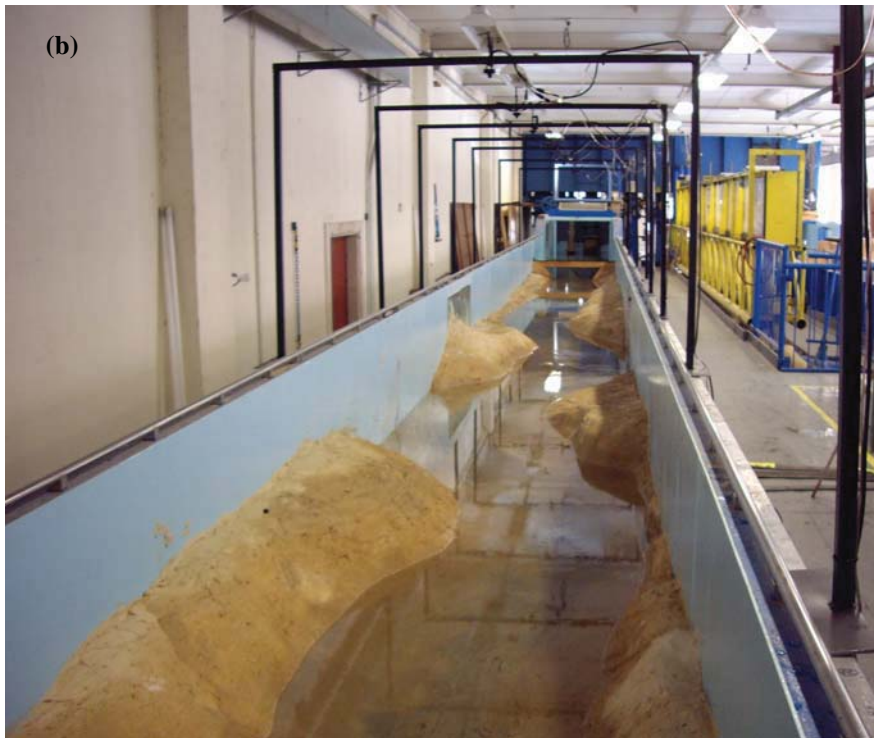
Figure 3.6: Photos of the flume, looking upstream (a) without water, showing the boulder piles and upstream wood pile, and (b) with water (low discharge), showing the cameras and camera frames.
