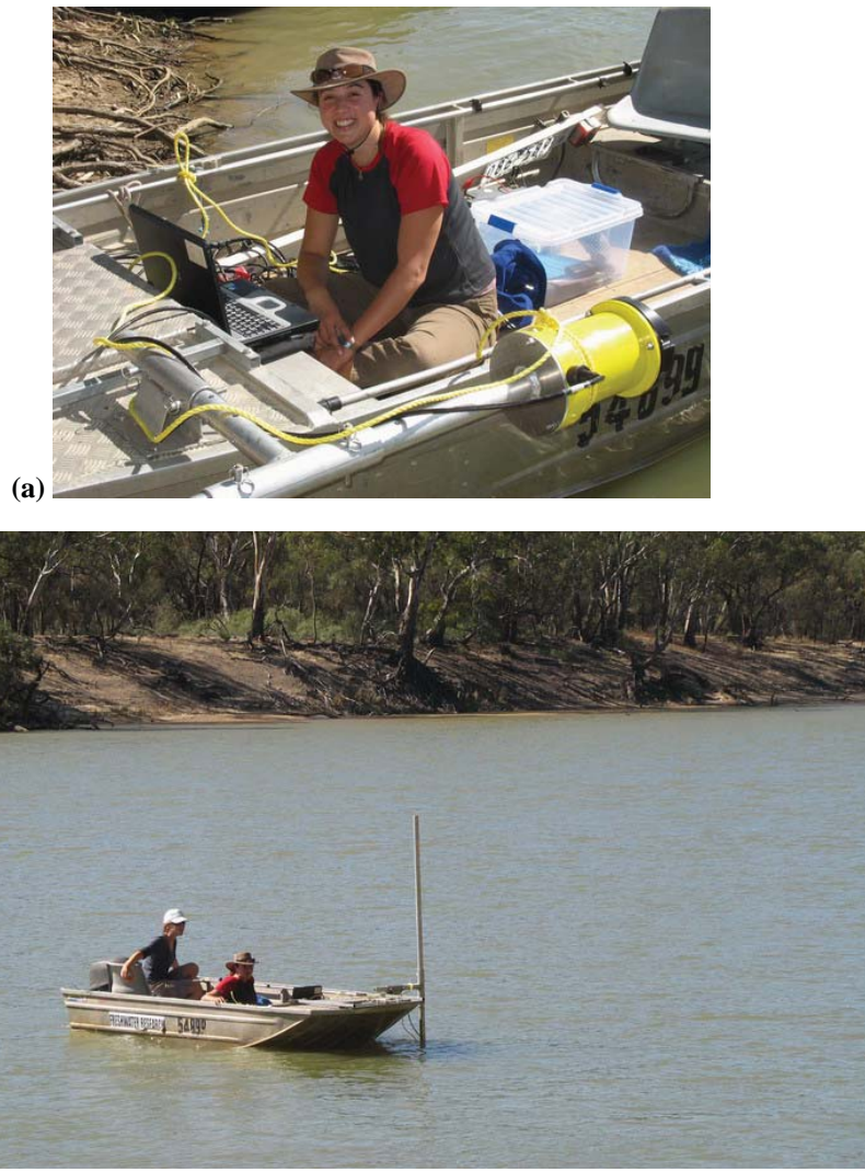
Figure 5.2: The boat-mounted, downward facing ADCP (a) set up and (b) in deployment.
