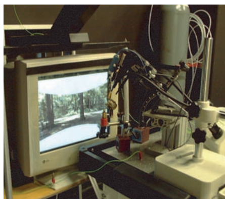
Figure 9.2. Electrophysiological experimental set up. Male hoverflies ( Eristalis tenax ) were positioned upright on a stand, which was mounted on a Newport anti-vibration recording table with a stimulus monitor in front of the fly. Naturalistic panoramic images were displayed on the inside of a virtual cylinder, which was centered on the fly and the perspective distorted according to the fly's calibrated 3D position and orientation relative to the screen. Motion simulated pure yaw rotations by spinning the virtual cylinder about a dorsal-ventral axis of the flies head. The display subtended approximately 90 degrees horizontally from the midline to the lateral portion of the animal, thus stimulating most of the receptive field of HS neuron.
